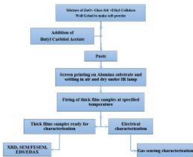
Fig. 1. Block Diagram of preparation and fabrication of thick film samples.
